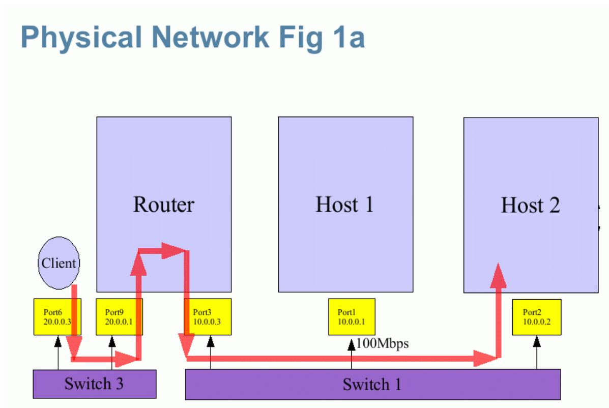
Lets take a physical network. The example in Fig 1a is representing the real network showing how my desktop connects to the Lab servers. The desktop is on 20.0.0.0/24 network while the server machines (host1 and host2) are on 10.0.0.0/24 network. In addition, host1 has got a 10/100 Mbps NIC limiting its connectivity to 100Mbps.
