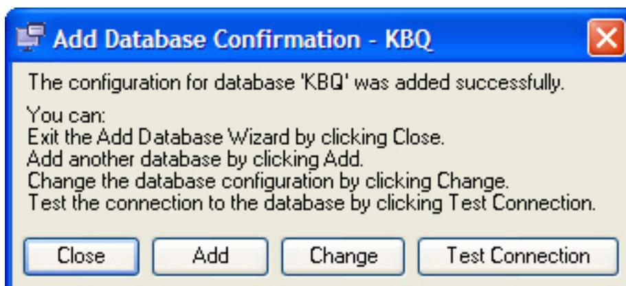
At this point, you can test the connection to make sure that the client can communicate with the database. If the test is successful, you can now use an application to access the DB2 database.
