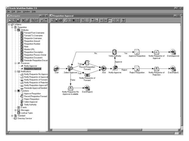
We refer to the whole drawing as a process or process diagram. The icons represent activities, and the arrows represent the transitions between the activities. In the above example, new items are created for the process when a user creates and submits a requisition in the appropriate application.
