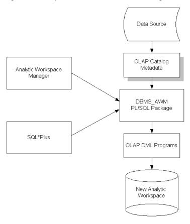
Figure 6–1 Components Used With the OLAP Catalog to Build an Analytic Workspace
