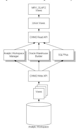
Figure 5–3 Tools for Creating Metadata for Analytic Workspaces
