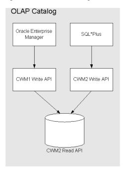
Figure 5–2 Tools for Creating OLAP Catalog Metadata for Source Data
