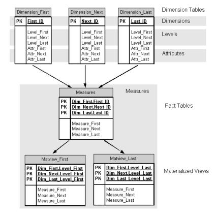
Figure 2-2 Diagram of a Star Schema
