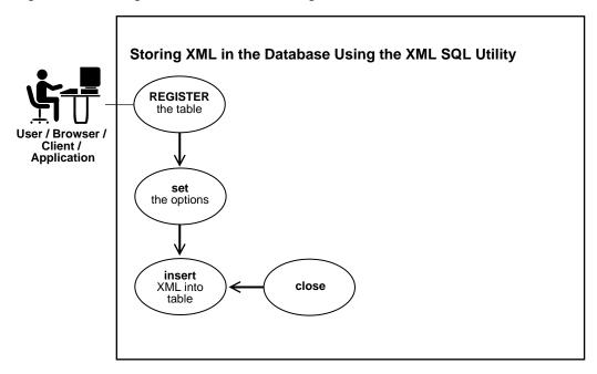
Figure 7–6 Storing XML in the Database Using XSU
