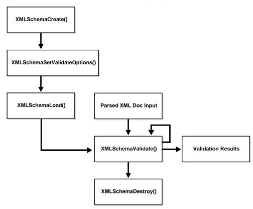
Figure 16–1 XML Schema Processor for C Usage Diagram
