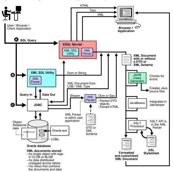
Figure 1–6 Generating XML Documents Using XDK Java Components
