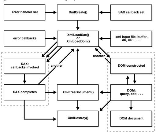
Figure 14-1 XML Parser for C Calling Sequence
