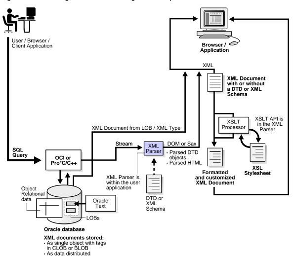
Figure 1–7 Generating XML Documents Using XDK C Components
