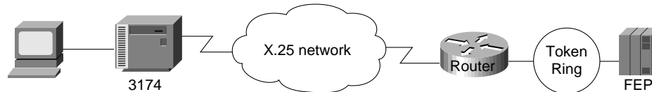
Figure 5-18 Simple topology for QLLC conversion.
