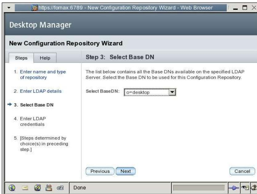
The screenshot shows the same web browser window, now at "Step 3: Select Base DN". The instructions state: "The list below contains all the Base DN's available on the specified LDAP Server. Select the Base DN to be used for this Configuration Repository." The left sidebar shows steps 1 through 5, with step 3 highlighted. The main form area contains a dropdown menu for "Select BaseDN:" with the value "o=desktop" selected. At the bottom, there are "Previous", "Next", and "Cancel" buttons.
