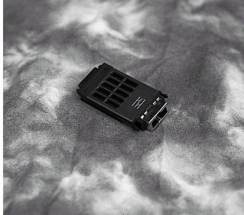
Figure 3-4. Active Copper GBIC (with HSSDC Connector)
