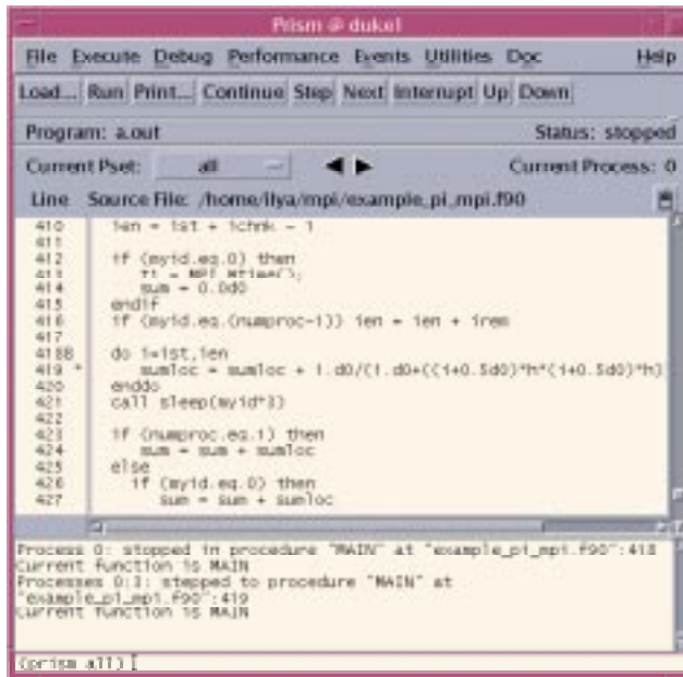
FIGURE 11-8 Debugging an MPI Application With Prism
