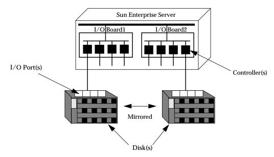
In this figure, the boot/root/swap disk and mirror have separate I/O buses, I/O boards, I/O controllers, I/O links, and I/O ports. Of course, they also exist on separate disks.
