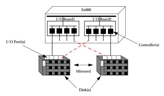
It requires care to successfully recover from a failure while the system is operating. Recovery procedures should be well defined and understood. If you replace any hardware that involves data I/O, the affected data bus must be in a quiescent state. This is important because system applications may share the same data path that the system disk uses.
