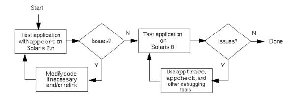
FIGURE 1 Using appcert, apptrace, and appcheck on Solaris  $^{\text{TM}}$  Operating Environment releases
