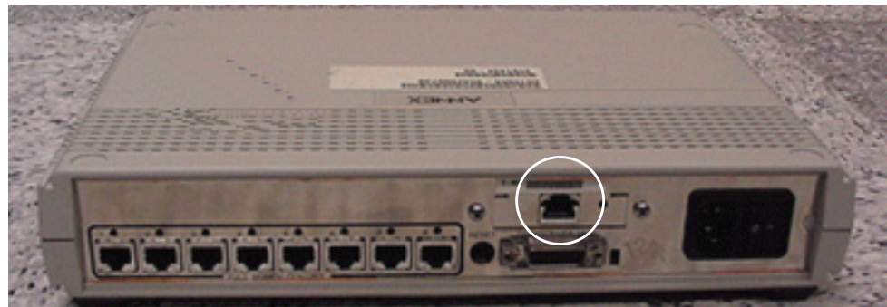
Figure 1-3 Typical 8 Port Terminal Concentrator (Rear view)—Ethernet Port Circled
