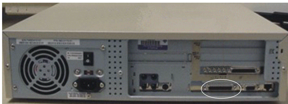
Figure 1-7 Ultra 5 Workstation Serial Port (Rear View)—Serial Port Circled
