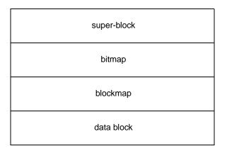
The super-block is similar to the super-block of a standard VxFS file system, but the magic number is different and many of the fields are not applicable.
