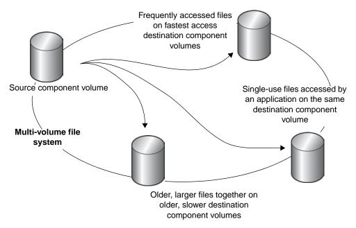
To use file relocation, you configure policies to determine the files to select for relocation. The fssweep utility traverses a directory structure applying selection rules from the configuration file, selects eligible files, then relocates the files from the source component volumes to destination component volumes.
