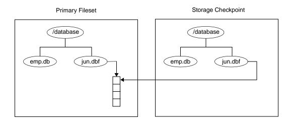
In the figure below, each block of the file system is represented by a square. Similar to the previous figure, this figure shows a Storage Checkpoint containing pointers to the primary fileset at the time the Storage Checkpoint is taken.
