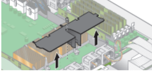
FIGURE 3 Removing the Center Air Baffle
