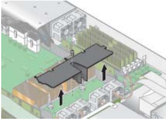
FIGURE 4-8 Removing the Center Air Baffle
