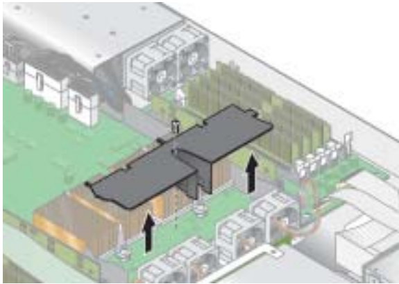
FIGURE 4-20 Removing the Center Air Baffle
