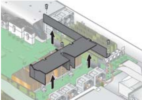
FIGURE 4-17 Removing the Center and Side Air Baffles
