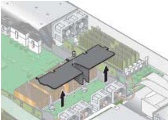
FIGURE 4-28 Removing the Center Air Baffle
