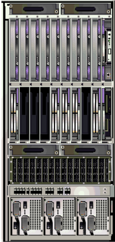
FIGURE 5-2 Sun Fire High-End Systems Platform Physical View—Front
