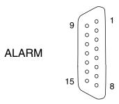
FIGURE 1 Alarm Port Pin Numbering
