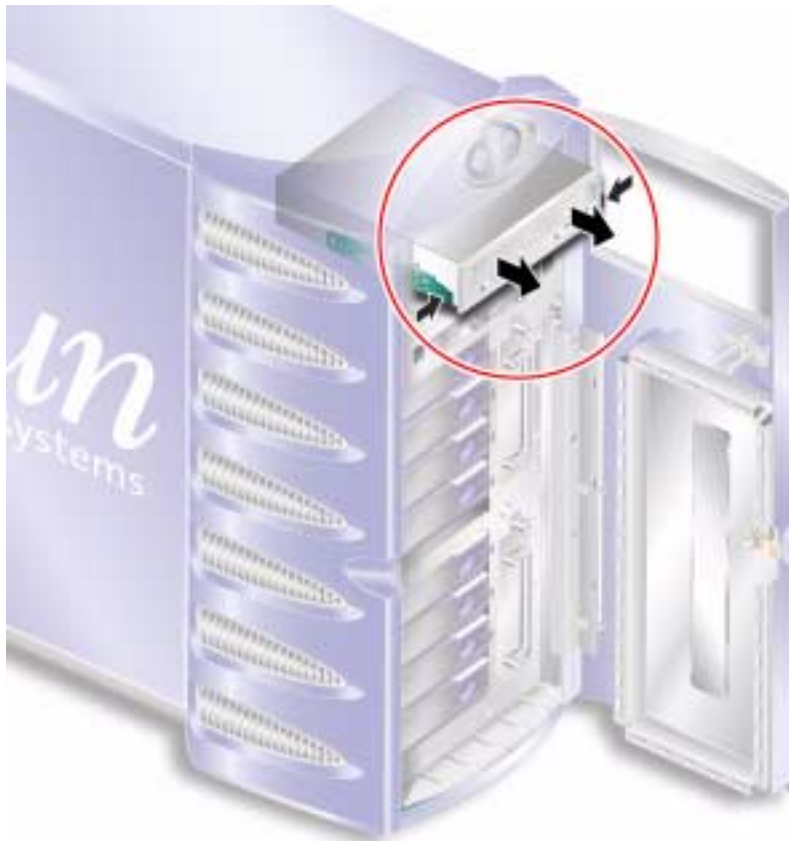
FIGURE 1-30 Removing the DVD-ROM Drive
