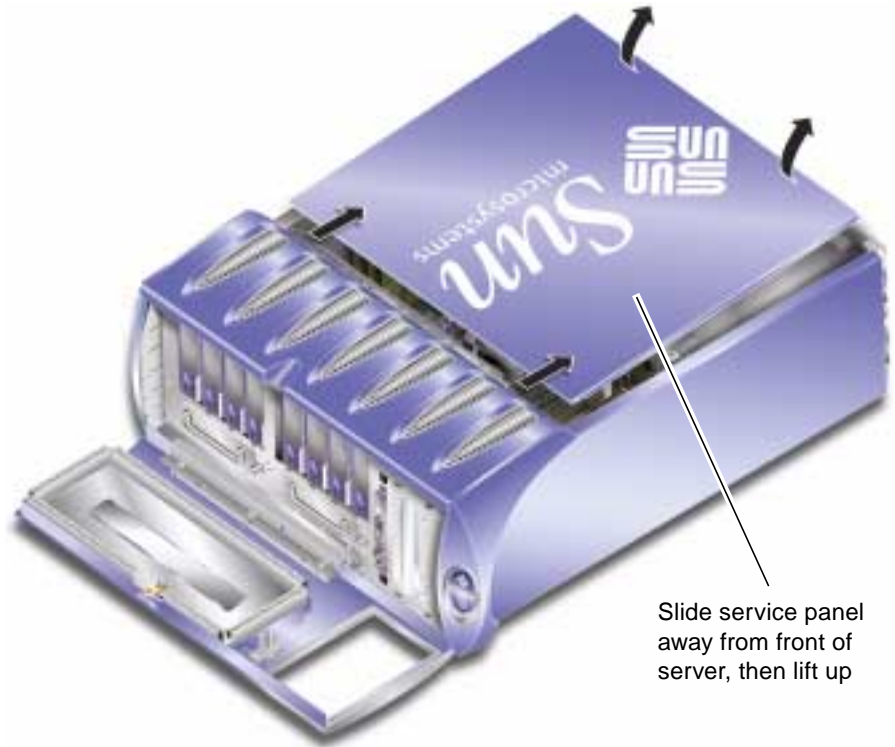
FIGURE 1-4 Removing the Service Panel
