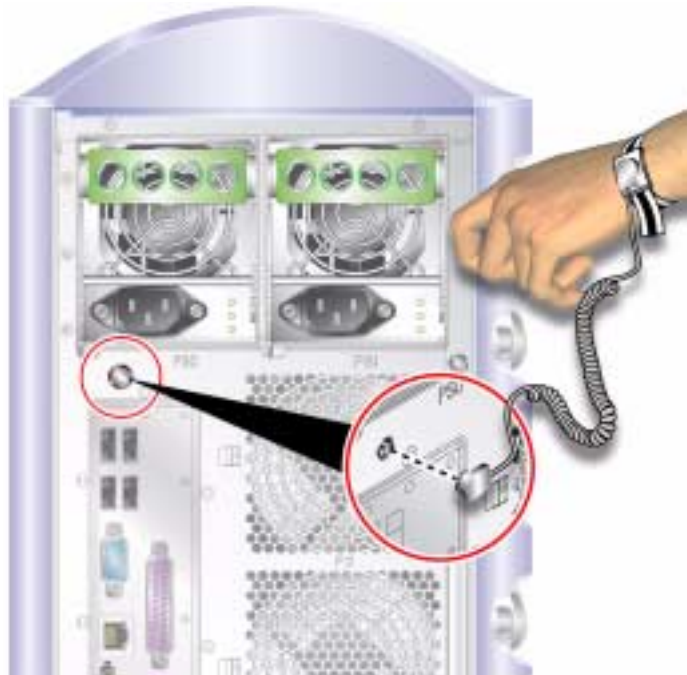
FIGURE 1-2 Back Panel Electrostatic Grounding Point
