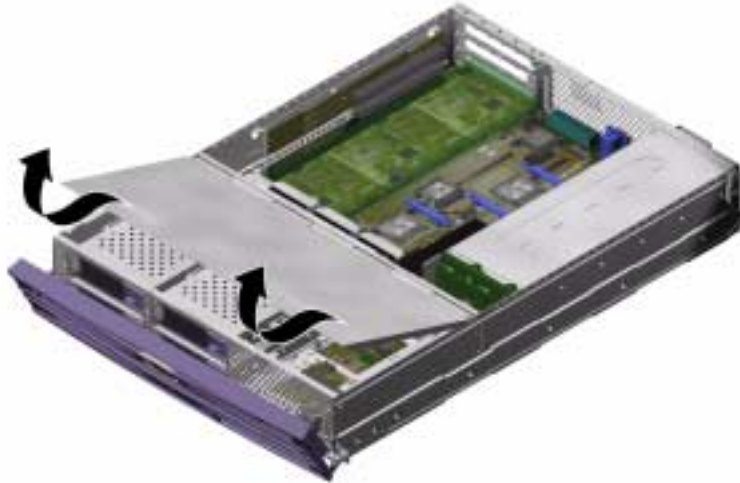
FIGURE 1-3 Removing the Front Section of the Lid
