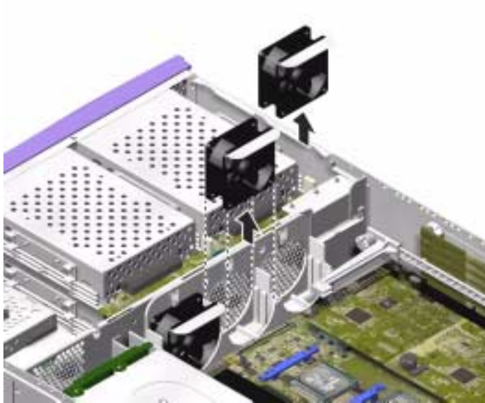
FIGURE 1-18 Removing Fans (Sun Fire V240 server shown)
