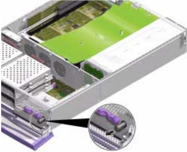
FIGURE 1-32 Removing the Keyswitch Assembly
