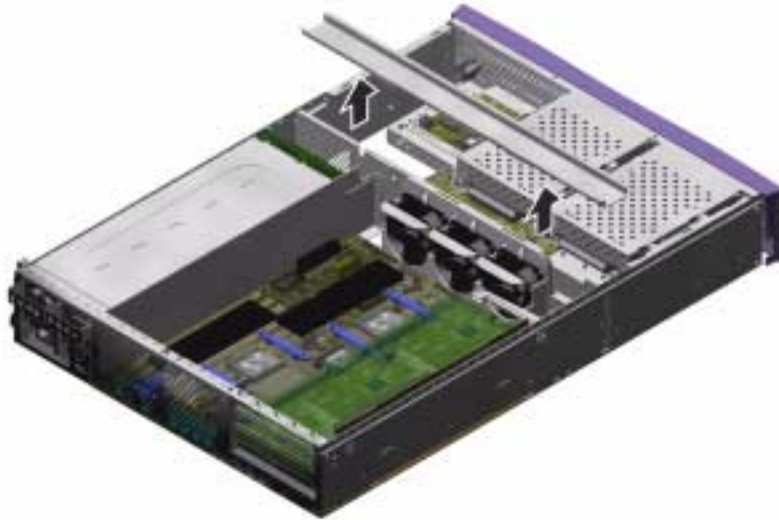
FIGURE 1-6 Removing the U-Channel
