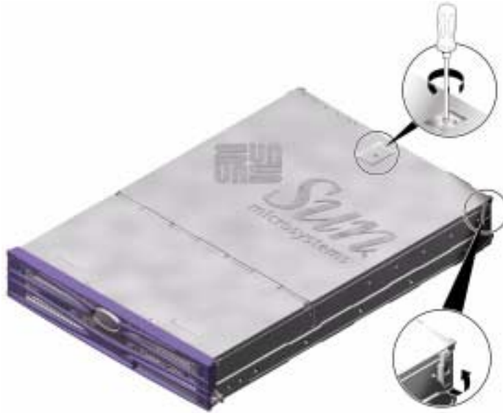
FIGURE 1-4 Location of Captive Screw and Side Catches on Back Section of Lid
