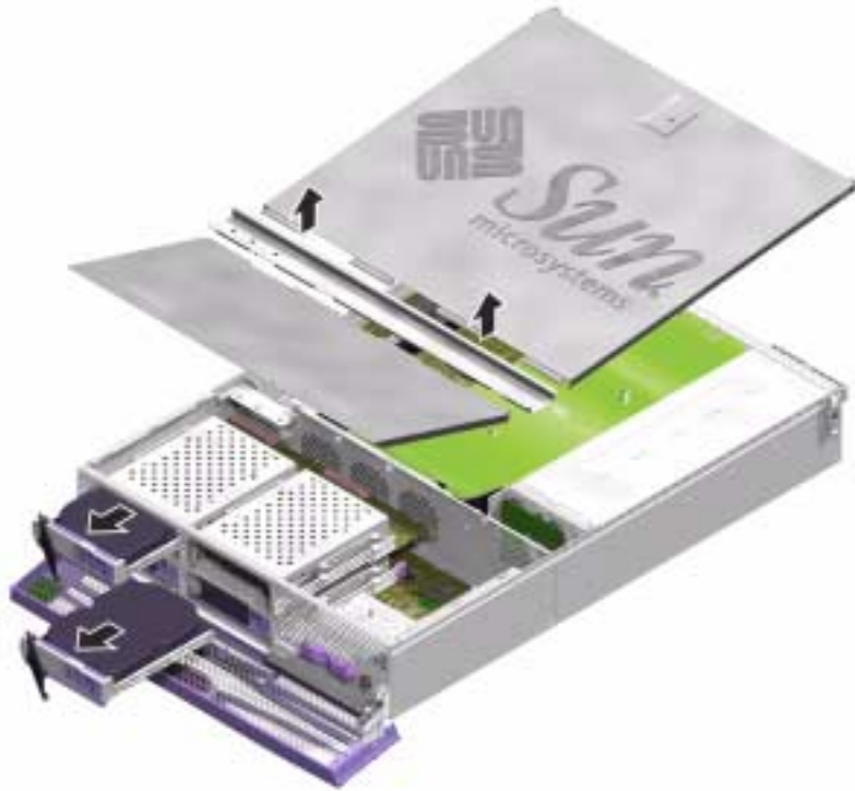
FIGURE 1-22 Removing Lid Assembly and Hard Disk Drives to Access Interface Boards
