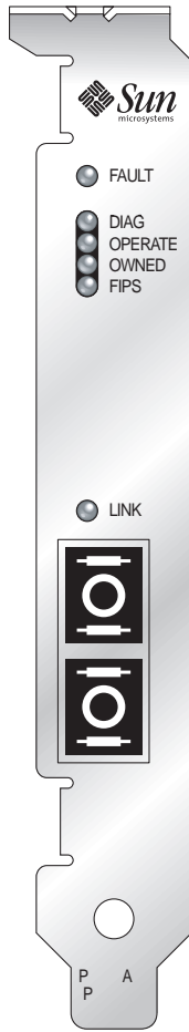
FIGURE A-1 Sun Crypto Accelerator 4000 MMF Adapter Connector
