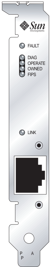
FIGURE A-2 Sun Crypto Accelerator 4000 UTP Adapter Connector
