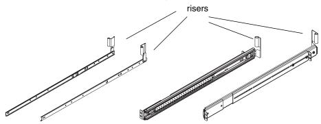
Install the inner glides and slide assemblies so that the risers point up. Each piece is labeled "LEFT" or "RIGHT" to indicate where it should be installed, as viewed from the front of the server.
