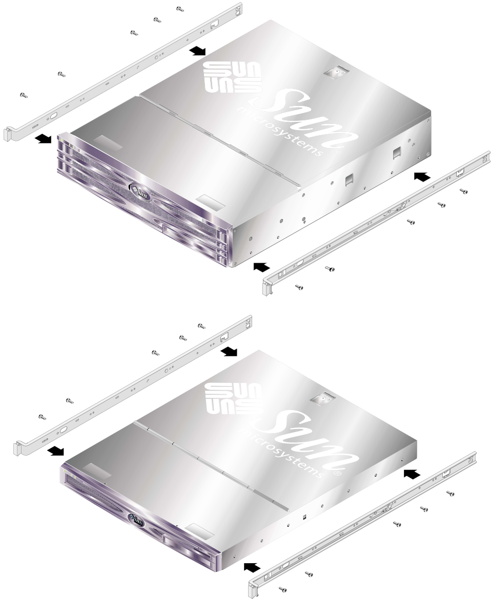
FIGURE 2-2 Attaching the Inner Glides to the Server
