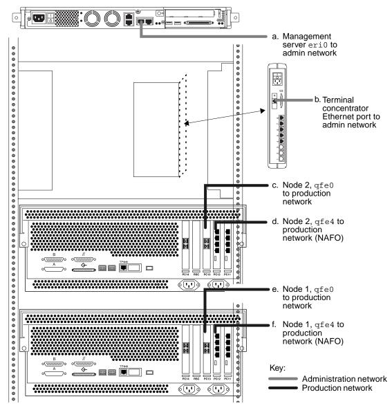
FIGURE 2-3 Clustered Database Platform 280/3 Connections to Your Networks
