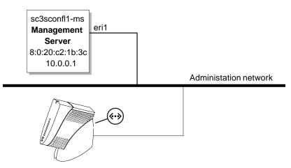
FIGURE F-1 Clustered Platform 280/3 Interconnections Using a Sun Ray Server
