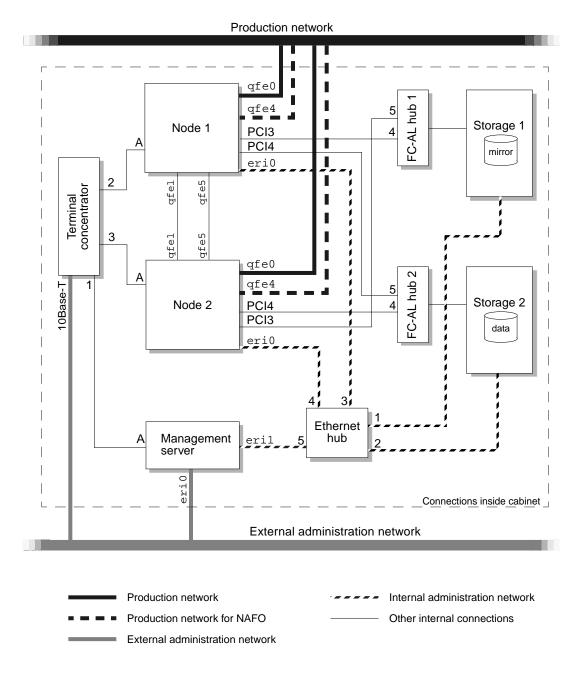
FIGURE 2-2 Clustered Platform Network Connections
