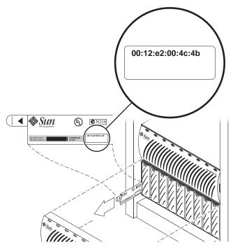
FIGURE 3-1 Location of Ethernet Address on Sun StorEdge Disk Array Pull Tab
