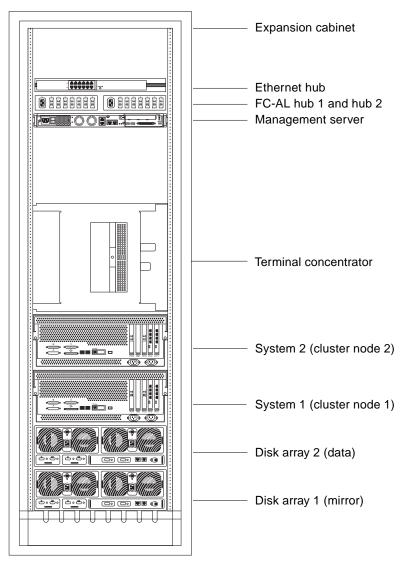
FIGURE 2-1 Clustered Platform Expansion Cabinet Placement
