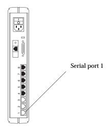
FIGURE 3-2 Terminal Concentrator Serial Port 1
