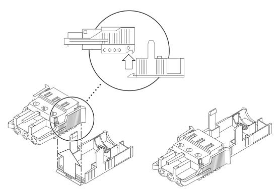
FIGURE 3-6 Inserting the Bottom Portion of the Strain Relief Housing
