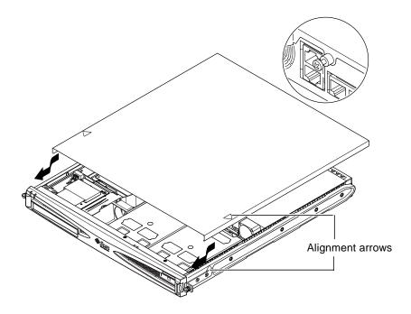
FIGURE 4-9 Replacing the Top Cover
