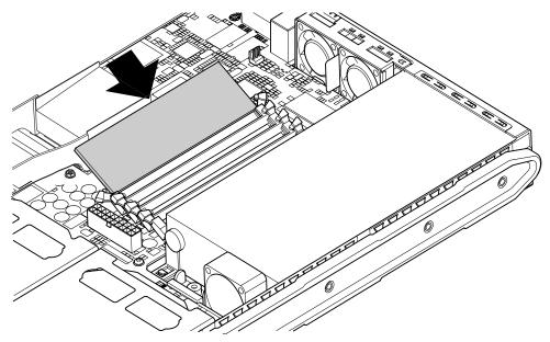
FIGURE 4-6 Installing Memory into a Socket on the System Board
