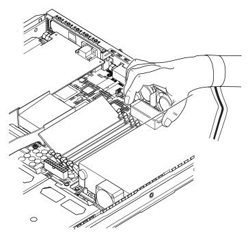
FIGURE 11-5 Replacing the NVRAM Chip
