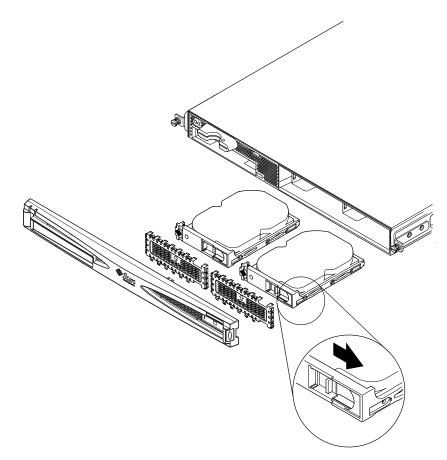
FIGURE 4-1 Inserting and Removing Hard Disks
