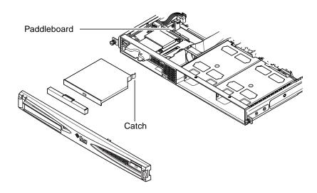
FIGURE 4-5 Installing an Internal DVD or CD-ROM Drive
