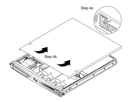
FIGURE 4-3 Removing the Top Cover
