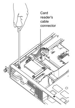
FIGURE 11-2 Removing the System Configuration Card Reader
