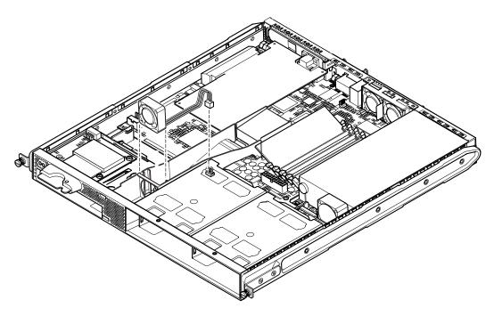
FIGURE 11-11 Disconnecting the Power Cable for Fan 3 and Lifting the Fan Out
