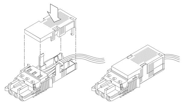
FIGURE 3-9 Assembling the Strain Relief Housing
