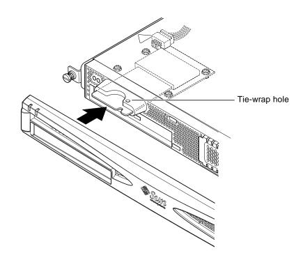
FIGURE 11-1 Replacing the System Configuration Card
