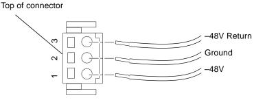
FIGURE 3-5 Assembling the DC Input Power Cable
