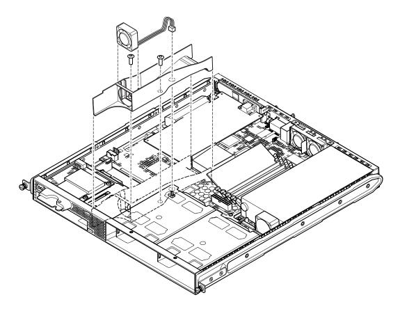
FIGURE 11-6 Unplugging and Removing the Fan 3 Assembly
