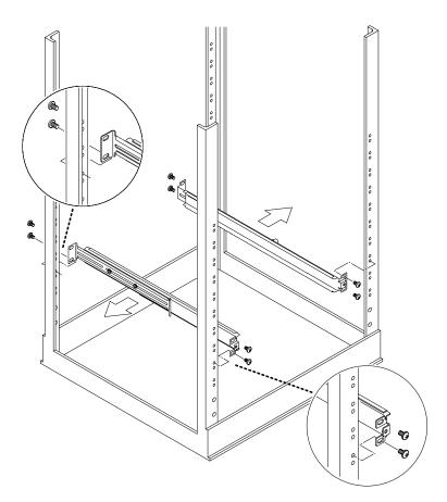
FIGURE 5-6 Fastening the Slide Mounts to a Standard 19-inch Rack
