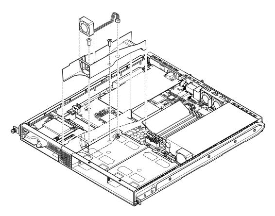
FIGURE 11-8 Replacing the Fan 3 Assembly
