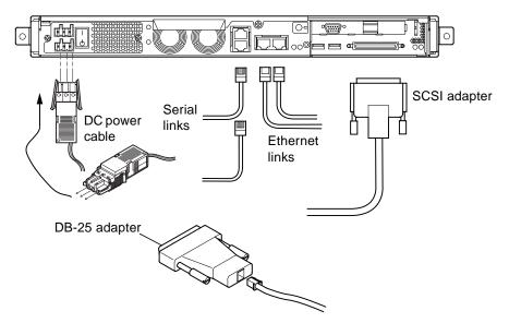
FIGURE 6-2 Connecting the Cables to the Netra 120 Server
