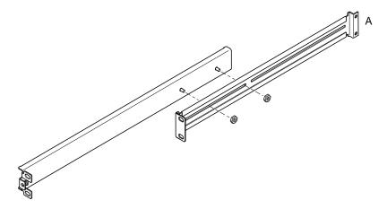
FIGURE 5-2 Positioning the Slide Mounts for a Sun StorEdge 72-Inch Tall Rack
