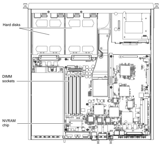
FIGURE 11-4 The Location of the NVRAM Chip
