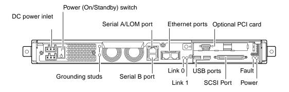
FIGURE 1-5 The Back Panel of the Netra 120 Server
