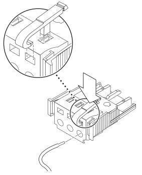
FIGURE 3-3 Opening the DC Connector Cage Clamp (Lever Method)
