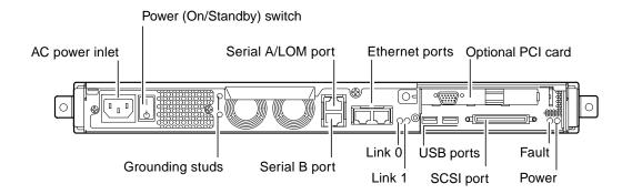
FIGURE 1-4 The Back Panel of the Sun Fire V120 Server
