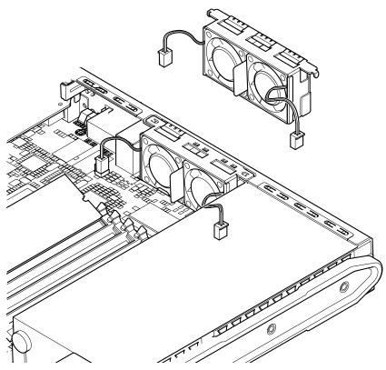
FIGURE 11-10 Replacing the Rear Fan Subassembly (Fans 1 and 2)
