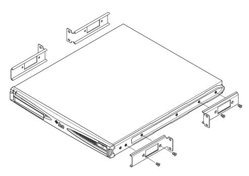
FIGURE 5-11 Fitting the Fixed Mounting Brackets
