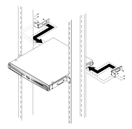
FIGURE 5-12 The Server Installed in a Two-Post Rack
