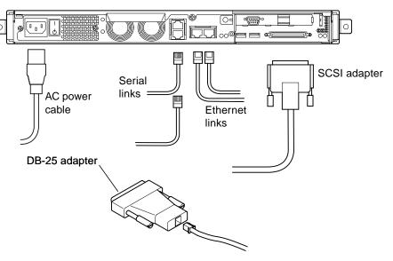
FIGURE 6-1 Connecting the Cables to the Sun Fire V120 Server
