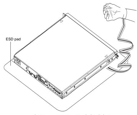
FIGURE 4-2 Using the Antistatic Wrist Strap Supplied With the Server
