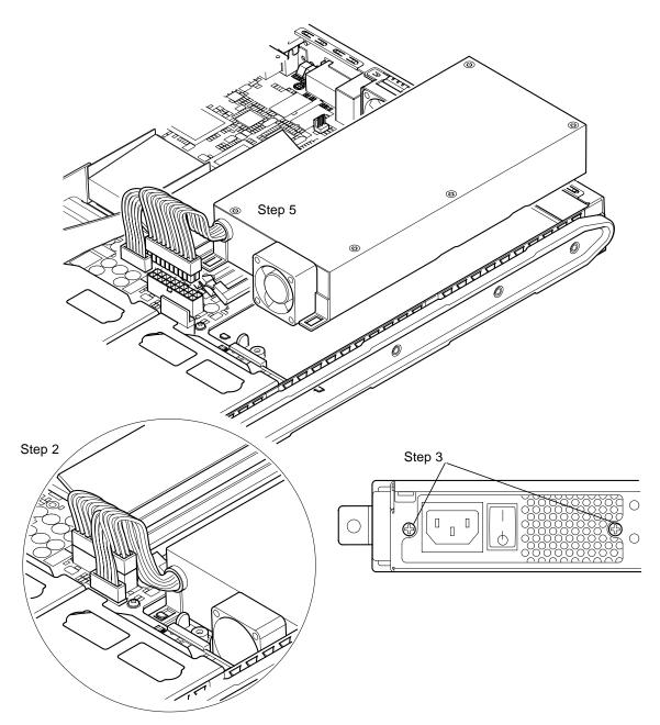
FIGURE 11-9 Replacing the Power Supply Unit
