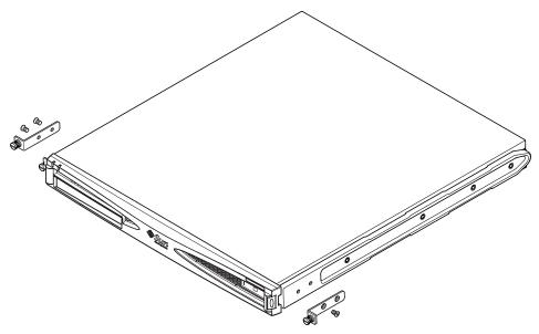
FIGURE 5-10 Removing the Thumbscrew Brackets
