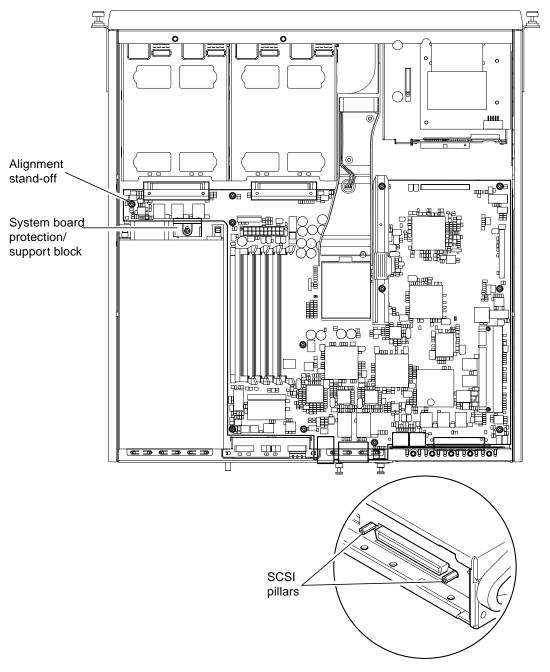
FIGURE 11-7 The System Board
