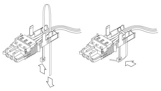
FIGURE 3-8 Securing the Wires to the Strain Relief Housing
