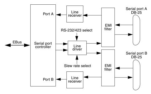
FIGURE 10-14 Serial Port Functional Block Diagram
