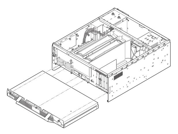
FIGURE 6-1 Power Supply Unit
