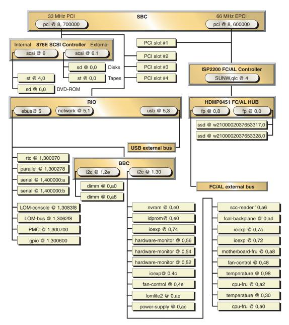
FIGURE 4-2 Netra 20 System Device Tree
