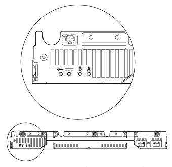
FIGURE 1-5 PSU Status LEDs (Netra 20 DC System)
