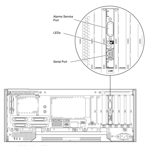
FIGURE 1-3 LOMLite2 Status LEDs
