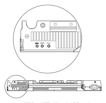
FIGURE 1-4 PSU Status LEDs (Netra 20 AC System)
