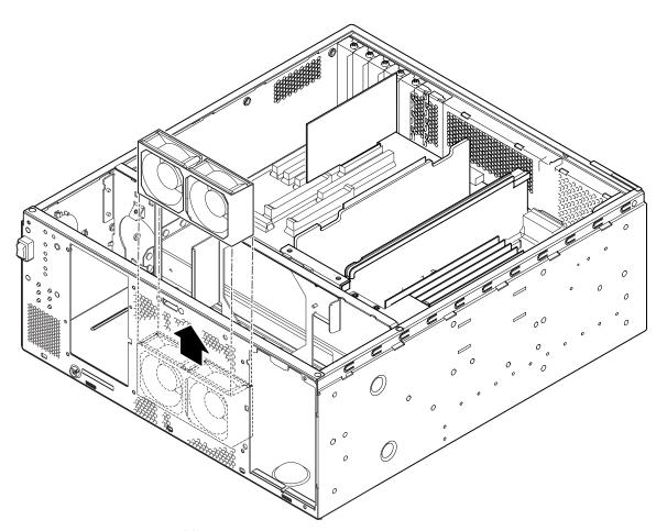
FIGURE 7-2 PSU Fans Assembly
