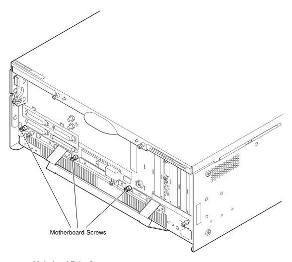
FIGURE 8-10 Motherboard Fixing Screws
