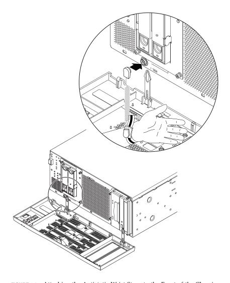
FIGURE 5-3 Attaching the Antistatic Wrist Strap to the Front of the Chassis
