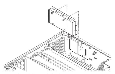
FIGURE 8-8 System Configuration Card Reader
