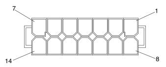
FIGURE D-5 Power Supply Connector J3601
