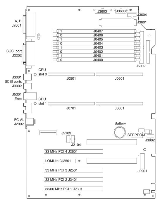
FIGURE 10-18 System Motherboard Block Diagram
