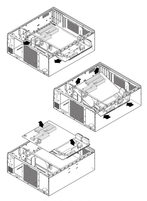
FIGURE 8-11 Removing the Motherboard from the Chassis
