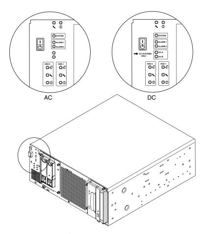
FIGURE 1-2 Front Panel System LEDs
