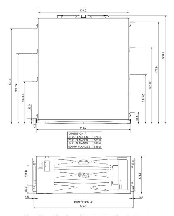
FIGURE 1-1 Netra 20 System Dimensions and Mounting Options (dimensions in mm)
