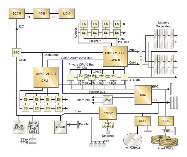
FIGURE 10-1 Netra 20 Logical System Diagram
