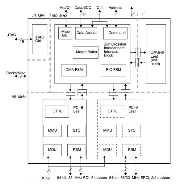
FIGURE 10-7 SBC Block Diagram
