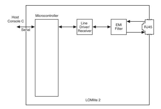
FIGURE 10-15 LOMlite2 Serial Port Functionality
