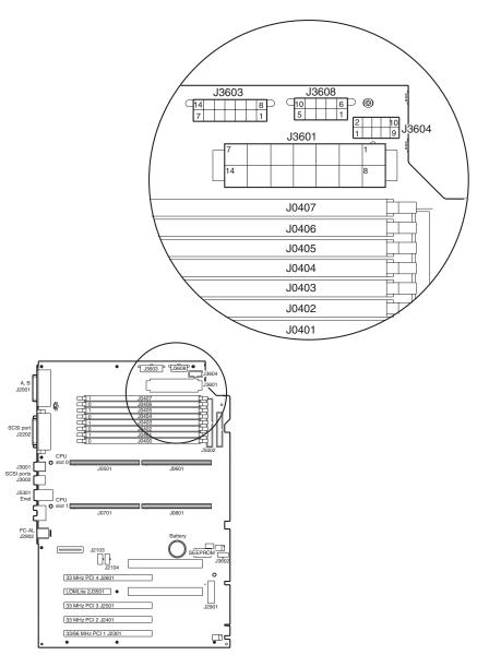
FIGURE 4-1 Power Supply Connector Jack Location
