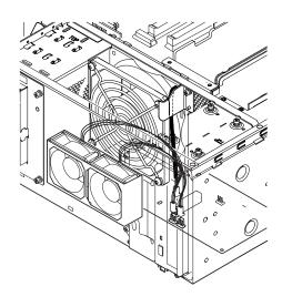
**FIGURE 7-4** Fan Connectors
