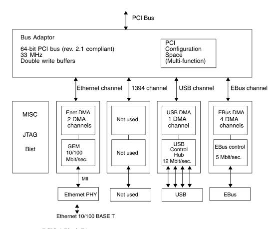
FIGURE 10-8 PCIO-2 Block Diagram
