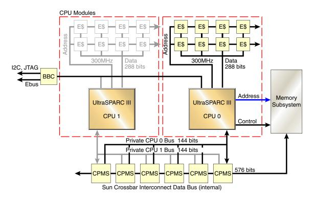
FIGURE 10-2 UltraSPARC-III Processor Functional Block Diagram
