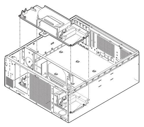
FIGURE 6-2 Power Distribution Board
