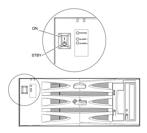
FIGURE 5-1 System Power On/STBY (Front Panel)
