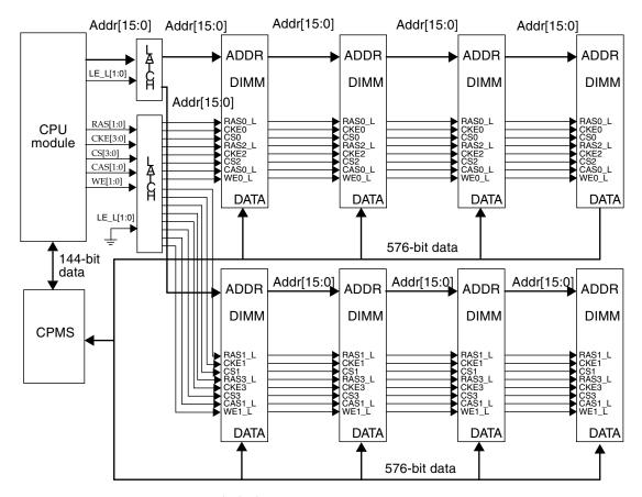
FIGURE 10-5 Main Memory Functional Block Diagram
