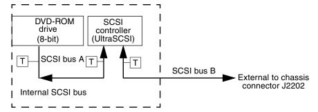
FIGURE 10-17 Configuration for the SCSI Bus
