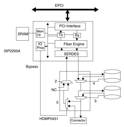
FIGURE 10-16 FC-AL Disk subsystem
