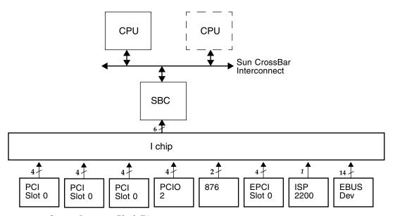
FIGURE 10-10 System Interrupt Block Diagram
