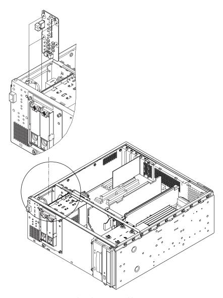
FIGURE 6-3 System Switch and LED Assembly
