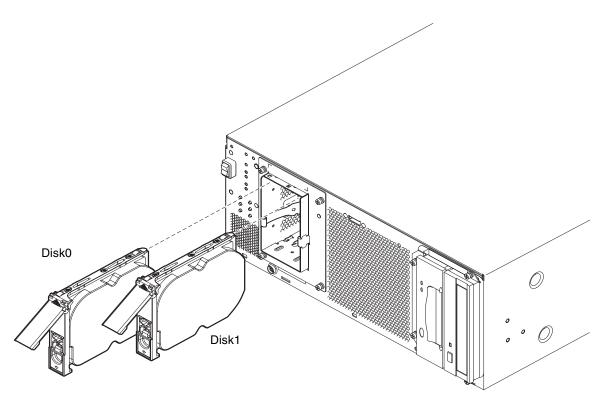
FIGURE 8-1 FC-AL Disk Drive and Drive Bay Assembly
