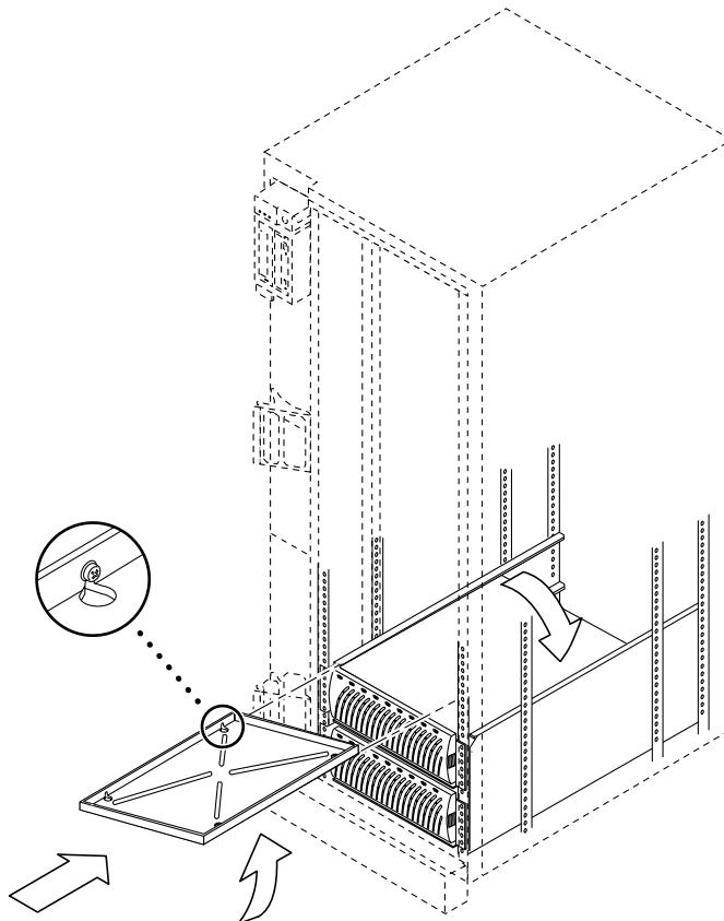
4. Tighten all four screws to secure the air baffle.
