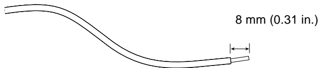
FIGURE 3-1 Stripping the Insulation From the Wire
