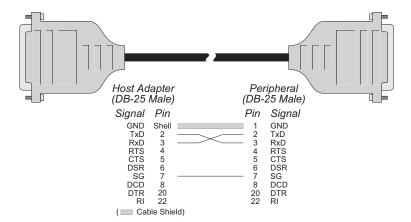
FIGURE 4-2 Simple Terminal/Printer Cable
