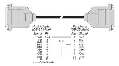
FIGURE 4-3 Terminal/Printer Cable with DTR Handshaking
