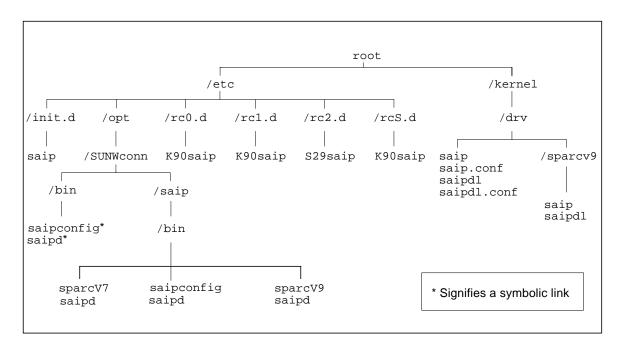
$\textbf{FIGURE 5-2} \quad SunSAI/P \; Software \; / \texttt{etc} \; and \; / \texttt{kernel Directory Structure for SAI/P 3.0}$
