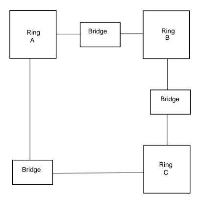
A disadvantage to this loop configuration is that each ring should be bridged to every ring on the network to for maximum performance and connectivity. Additionally, loop configurations are difficult and expensive to expand. To add one more ring to the loop configuration shown above, would require the addition of three more bridges. See the diagram below.
