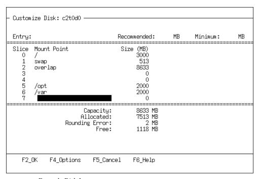
FIGURE 3-1 Example Disk Layout
