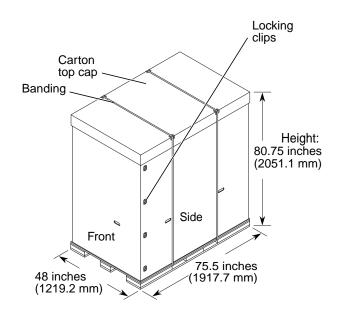
5. Remove outer cartons. Remove the hardware box located at the front or rear of the system and the two shipping kit boxes located on the sides of the pallet deck. Take out the 9/16-inch open-end wrench from the hardware box, and retain the remaining items for later use as needed.
