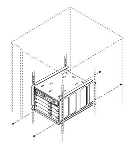
5. Secure the base plate to the side rails with four 10-32 x 1/2 inch screws, two screws at the front and two screws at the rear.
