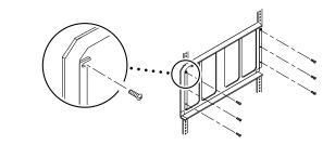
d. Install the four remaining screws, then tighten all six screws.
