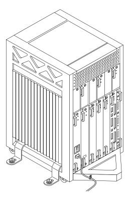
4. Insert and tighten the bolts through the holes on both ends of the brackets into the holes in the floor on each side of the system.
