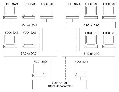
Figure 8-5 Hierarchical Tree of Concentrators
