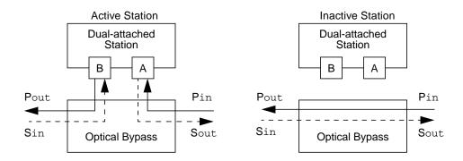
Figure 7-12 Optical Bypass Switch
