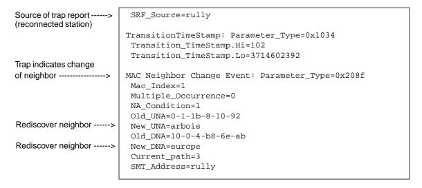
Figure 10-9 Dual-Attached Station Restarted
