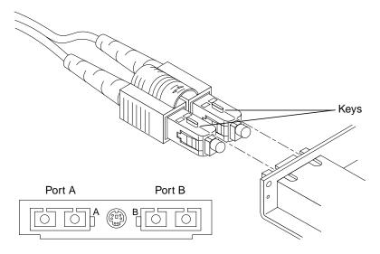
Figure 2-2 Aligning SC Type Fiber Optic Cable Connectors
