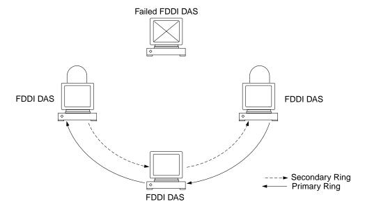
Figure 7-8 Isolating a Single Station Failure
