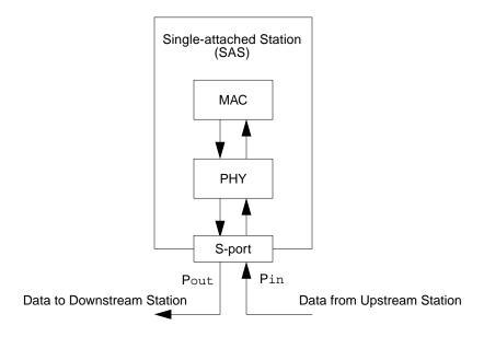
Figure 7-4 Single-Attached Station (SAS)
