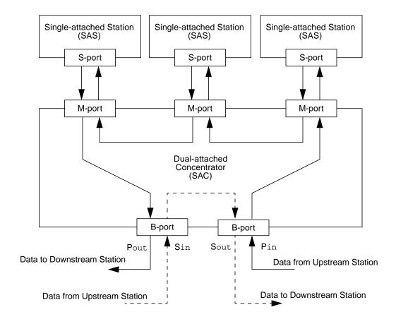
Figure 7-7 Dual-Attached Concentrator (DAC)
