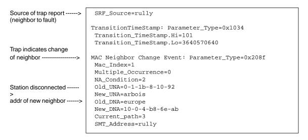
Figure 10-6 Single-Attached Station Disconnected
