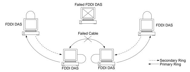
Figure 8-2 Basic Dual Ring Network with Two Faults
