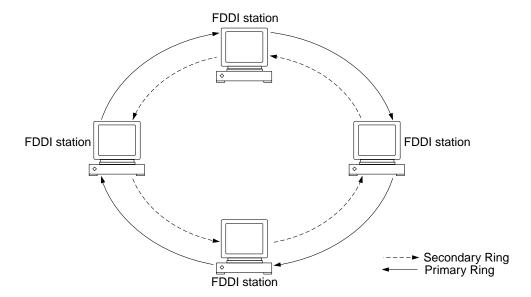
Figure 7-3 Basic FDDI Network Architecture
