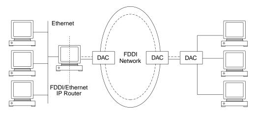
Figure 8-9 Ring of Trees Attached to an Ethernet Network
