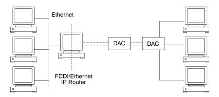
Figure 8-8 Tree of Concentrators Attached to an Ethernet Network
