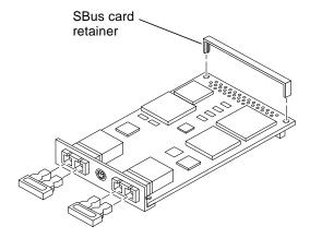
Figure 2-1 Removing Plastic Retainer From Rear of Card
