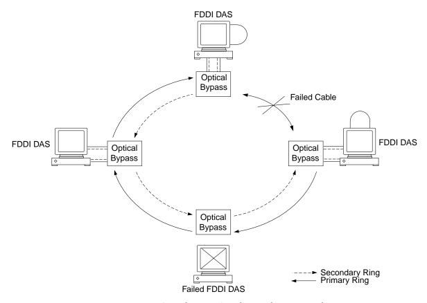
Figure 7-13 Optical Bypass Switches used in a Network
