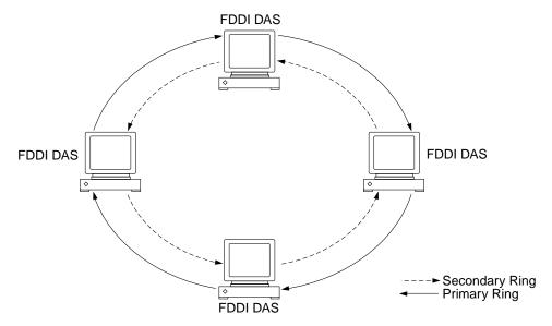
Figure 8-1 Basic Dual-Ring Network
