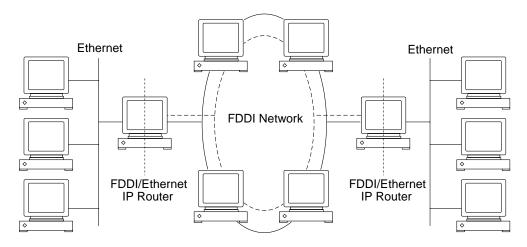
Figure 8-7 Basic Mixed FDDI/Ethernet Topology
