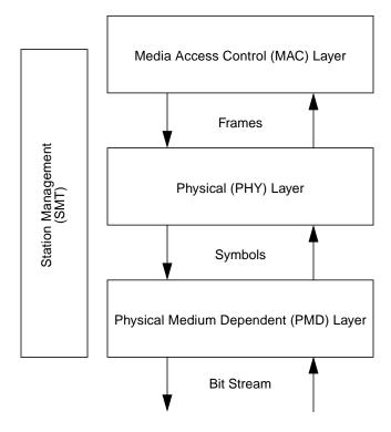
Figure 7-2 Communication Between FDDI Layers
