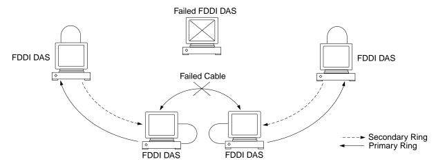
Figure 7-11 Dual Ring Network Divided by Two Faults
