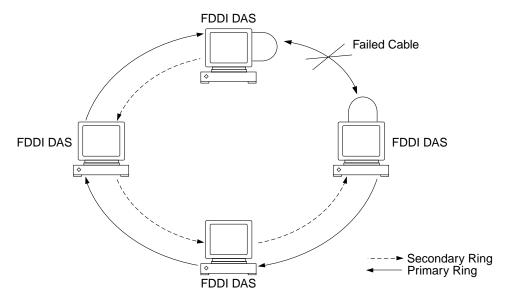
Figure 7-9 Isolating a Single Cable Failure
