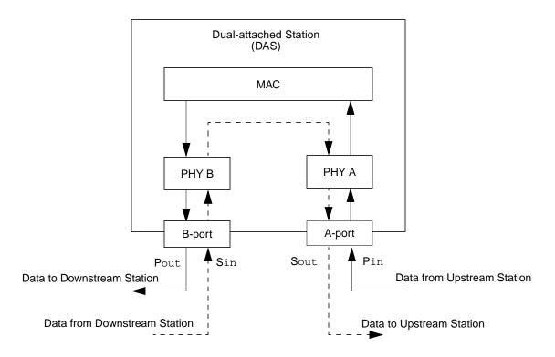
Figure 7-5 Dual-Attached Station (DAS)
