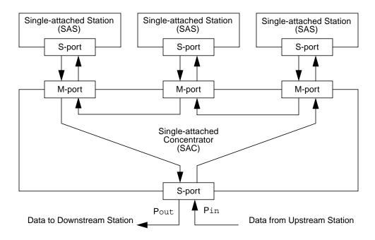
Figure 7-6 Single-Attached Concentrator (SAC)
