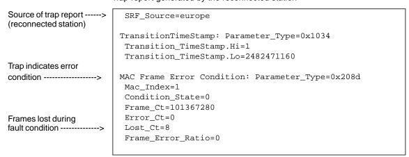
Figure 10-7 Single-Attached Station Reconnected
