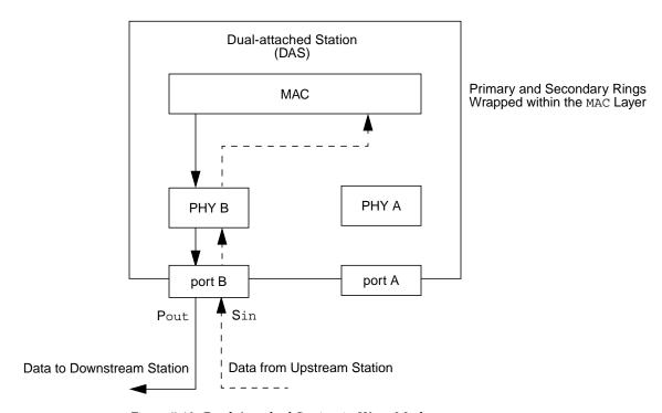
Figure 7-10 Dual-Attached Station in Wrap Mode
