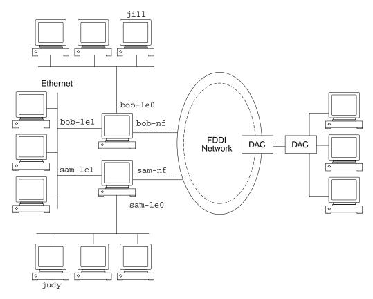
Figure 8-10 Routing in an FDDI/Ethernet Internetwork
