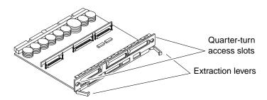
3. Pull the ends of both extraction levers toward you, then pull the board out of the card cage.
