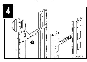
**IMPORTANT:** The mounting bracket must be parallel from front to rear before you secure it to the rack. The left and right mounting brackets must be parallel.
