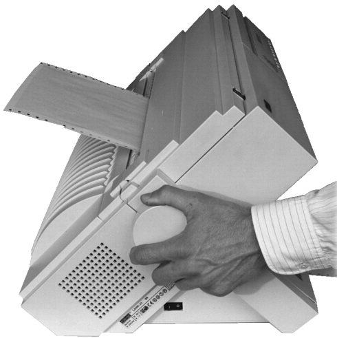
Moving the Paper with the Platen Knob
