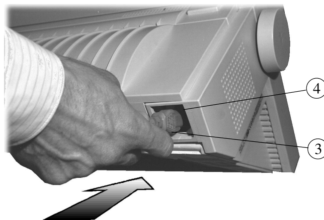
Plugging the Power Cable
