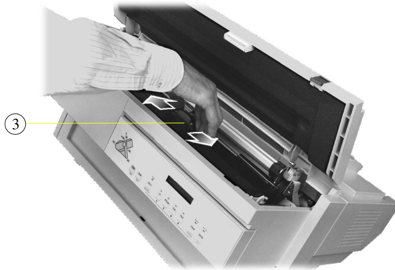
Checking the Ribbon Cartridge Installation
