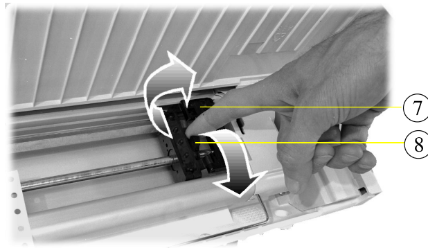
Unlocking the Right Tractor
