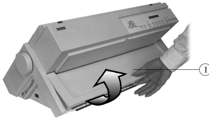
Opening the Front Slot Cover
