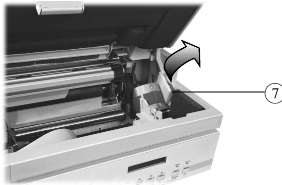
Removing the Carriage Motor Shipment Lock
