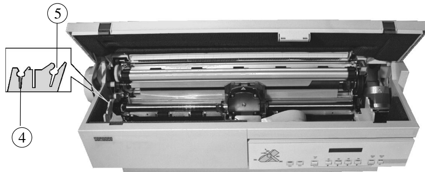
Aligning the Cartridge Pins with the Cartridge Supports
