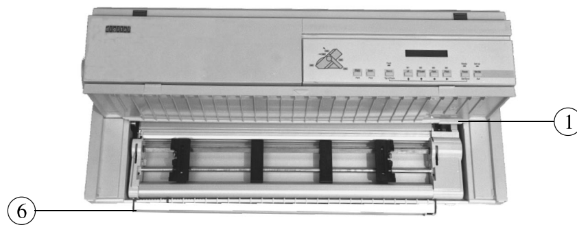
Mounting and Aligning the Push Tractor Unit in its Place
