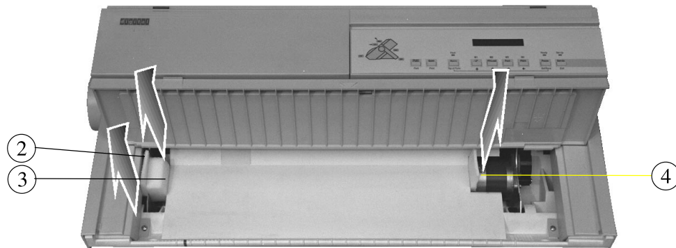
Removing the Basic Assembly Shipment Locks
