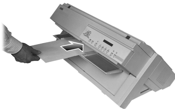
Inserting the Cut Sheet
