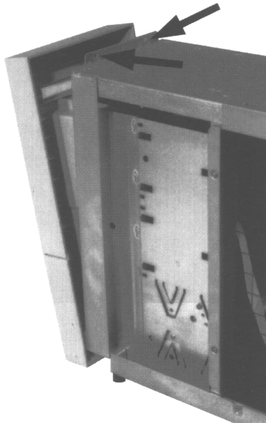
Figure 5-7 Front Bezel Mounting Screws
