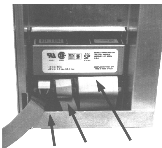
Figure 5-15 Drive Cable Connections – 1 drive version
