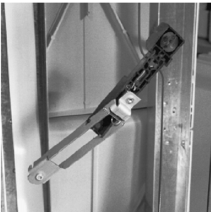
Figure 5–35 Positioning the Tensioner to Mount on Translate Frame
