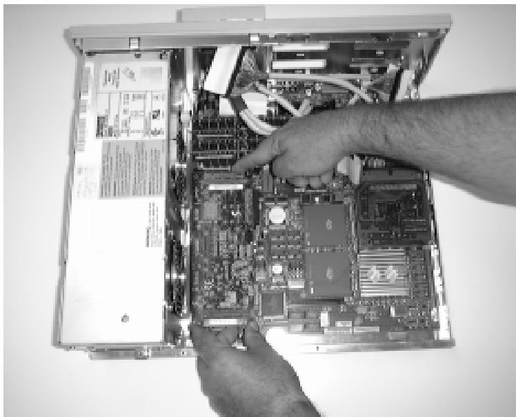
Figure 3 Installing the VAX-SCSI module
