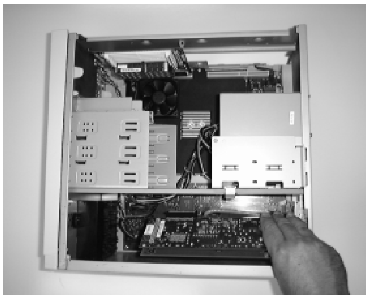
Figure 15: Installing the DS-KZCCA-DB VAX™-SCSI Adapter
