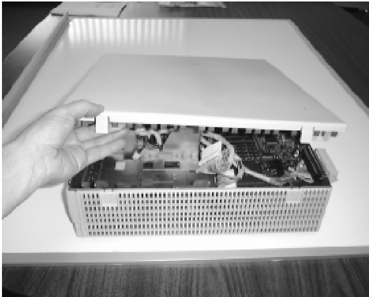
Figure 6: Accessing the VAXStation CPU
