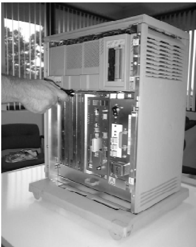
Figure 10: Accessing the CPU Module
