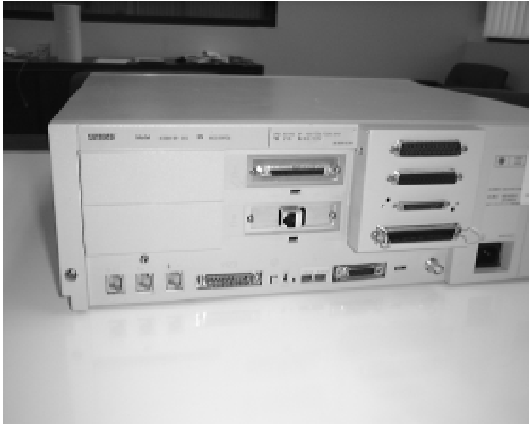
Figure 5: I/O Bulkhead installed
