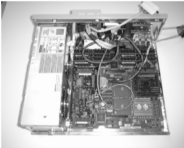
Figure 4: Routing the internal cables.
