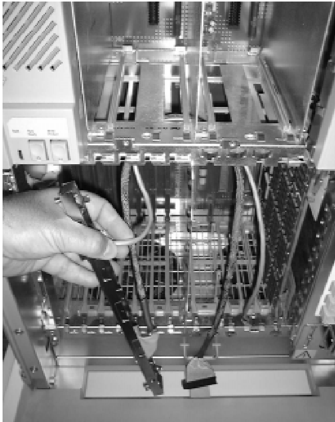
Figure 11 Routing the Cables
