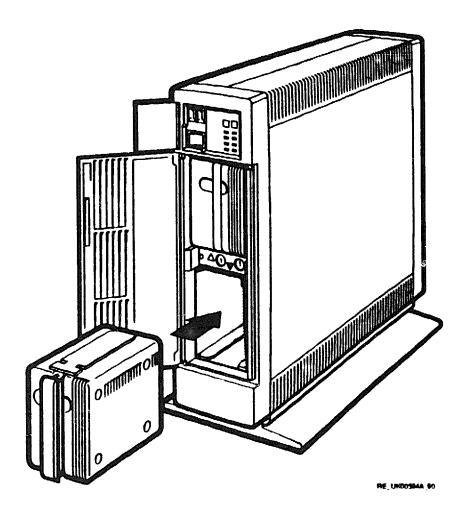
Figure 3-2 Inserting an RSD
