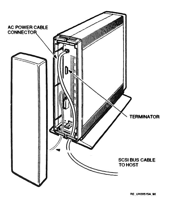
Figure B-2 Cabling the Pedestal
