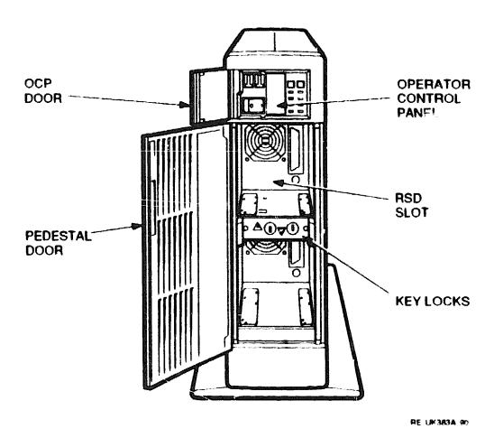
Figure 1-1 Front View of R23RZ Pedestal with Canisters Removed
