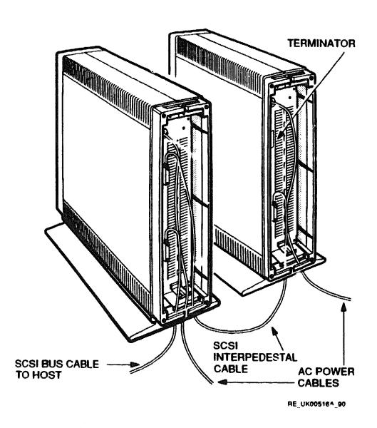
Figure B-3 Interpedestal Cabling
