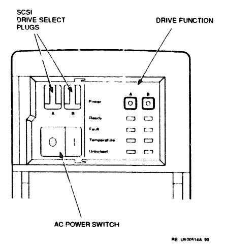
Figure 3-1 Operator Control Panel (OCP)
