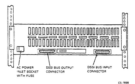
Figure B-3 Rear View of R23RF-C Rackmount Disk System
