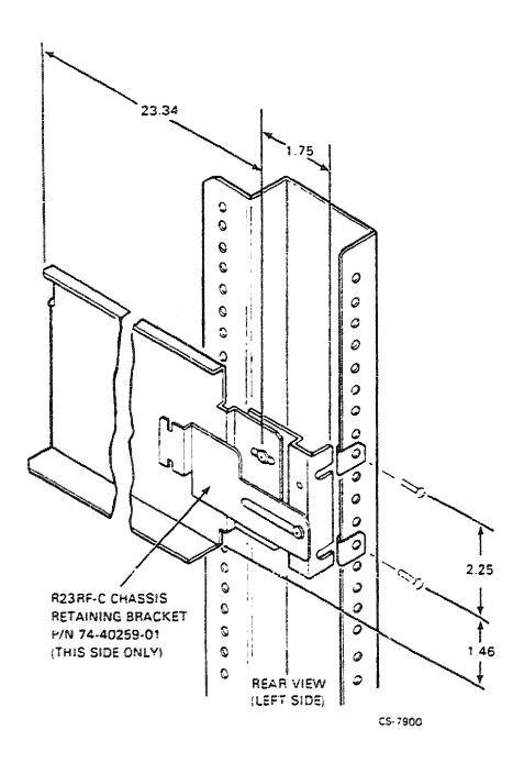
Figure B-1 Rackmount Disk System Dimensions
