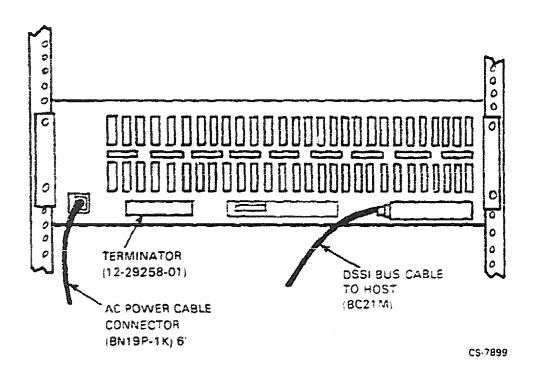
Figure B-4 Cabling the Rackmount Disk System
