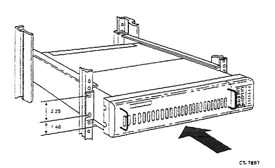
Figure B-2 Inserting the Disk System in the Rackmount
