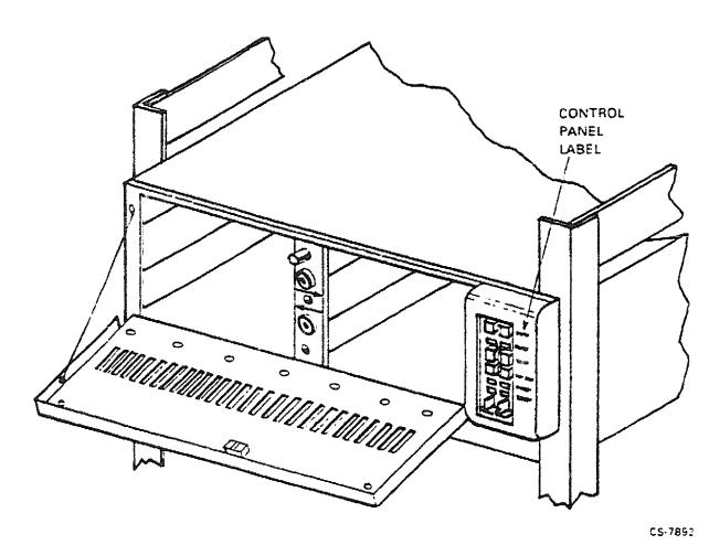
Figure 1–1 Front View of R23RF-C Rackmount Disk with RSEs Removed
