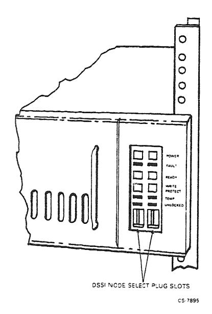
Figure 3-1 Operator Control Panel
