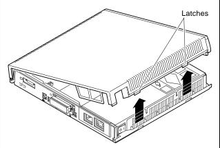
Caution: You may damage the equipment if you do not wear an antistatic wrist strap when working inside the system unit.
